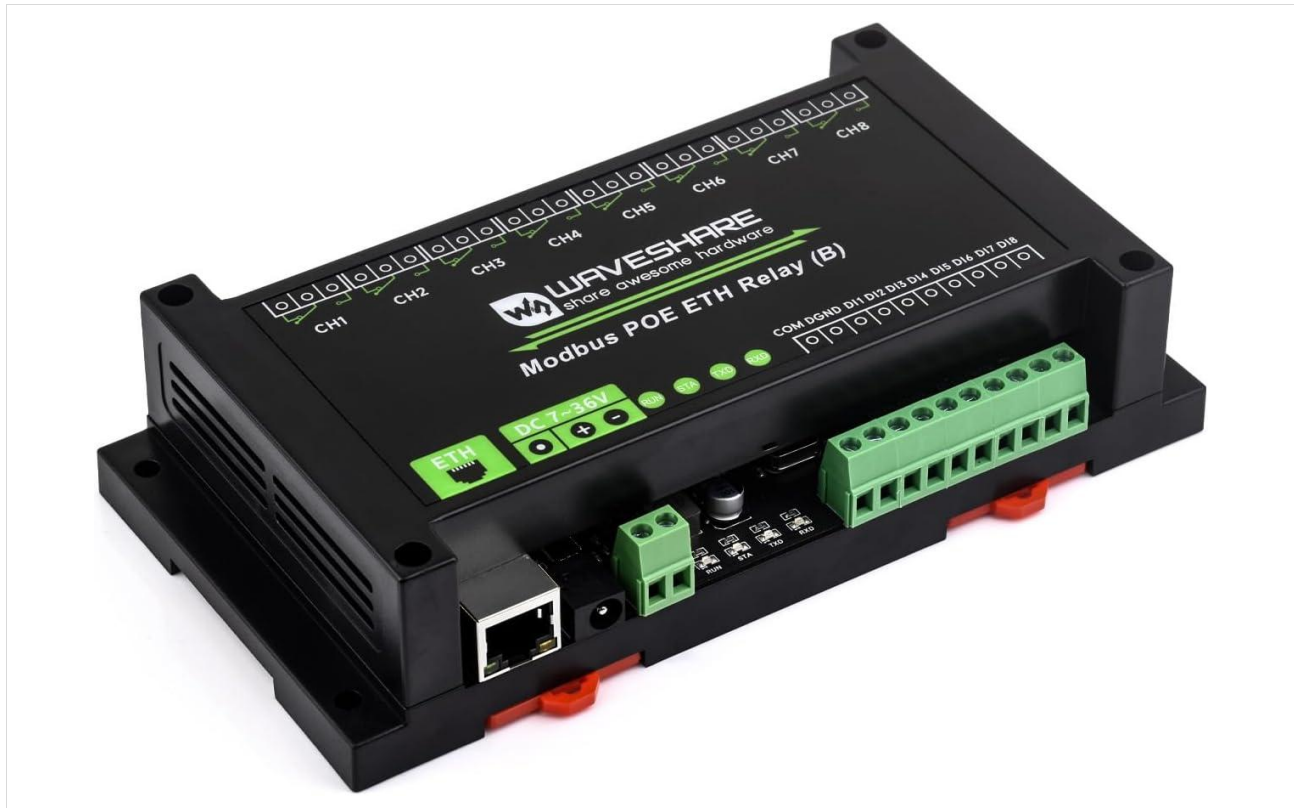
Figure 1 — WAVESHARE Modbus POE ETH Relay (B) module. You can see the Ethernet port (ETH), the DC 7~36V power input, the RUN/STATX/D/RXD indicators and the 8 relay channels (CH1 to CH8).
